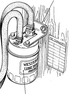
APPLY A THIN COAT OF CLEAN OIL TO THE FILTER GASKET WHEN INSTALLING. WHEN THE FILTER CONTACTS THE BASE, TIGHTEN IT (BY HAND) A 3/4 TURN MORE.
