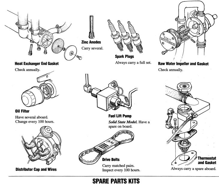
WESTERBEKE also offers two Spare Parts Kits, each packaged in a rugged hinged toolbox. Kit A includes the basic spares. Kit B is for more extensive off-shore cruising.
