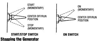
To stop the generator, move the momentary START/STOP switch to the down (*stop*) position then release it to the center (*off/run* mode) position. This will activate the remote control panel for START/STOP functions.
