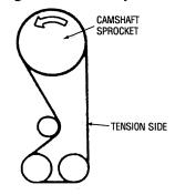
7. Loosen the temperorarily tightened tensioner nut on the water pump side 1 or 2 turns, and tension the belt making use of spring force.
