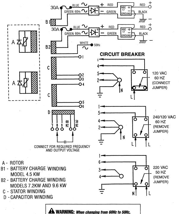
**ACA WARNING:** when changing from 60HZ to 50HZ, make certain the ground wire (white & green stripe) is properly repositioned according to this diagram.
