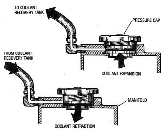
After checking for leaks, stop the engine and allow it to cool. Coolant should drain back into the cooling system as the engine cools down. Add coolant to the recovery tank if needed. Clean up any spilled coolant.
